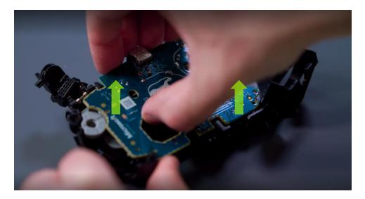
Procedure – Installation (I/O Board)
